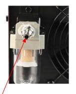
3. Connect the air supply to the air connection located at the rear of the machine. Turn on the air supply.
