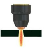
Torch height too low, reverse bevel. Tip may contact the work piece and short out or damage the tip.
