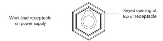
Push the work lead connector all the way into the receptacle on the power supply and turn clockwise, approximately 1/4 turn, until the connector is fully seated against the stop in order to achieve an optimal electrical connection.
