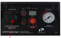
6. Set the amperage dial Set the air pressure at 60-70PSI
