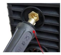
2. Connect the earth lead to the output terminal of the machine and Tighten
