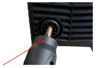
Connect the IPT60 Plasma torch to the machine. Ir the torch connection into the torch connection recept the front of the machine and fasten tightly. Caution: Do not to bend the pins located inside the torch
