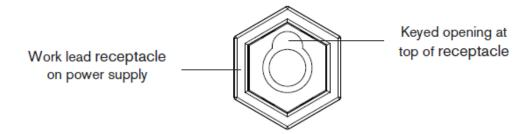
Push the work lead connector all the way into the receptacle on the power supply and turn clockwise, approximately 1/4 turn, until the connector is fully seated against the stop in order to achieve an optimal electrical connection.
