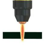
Torch height too high excessive bevel, plasma Stream may not cut all the way through the material.
