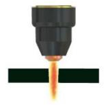
Correct torch height and square to the material, minimum bevel & equal bevel gives the longest consumable life.
